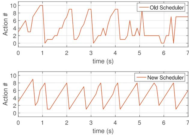
Fig. 7. Action sequences for the bongo board task with a heavy object on the character’s left arm. Top: The scheduler learned on the normal character is used. Bottom: The scheduler is learned for this new task.
