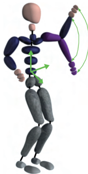
Fig. 8. The body configuration parameters are a set of joint positions in the root segment coordinate system of the human body. They are concatenated to form a vector in high dimension space. The L2 distance metric is used in the clustering.
