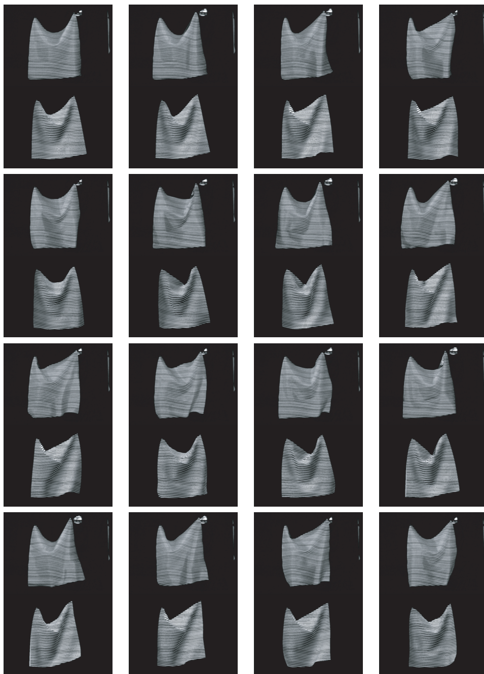
Figure 2.17: Waving results for satin. The top picture in each block shows the real fabric and the bottom shows the corresponding frame from simulation.
