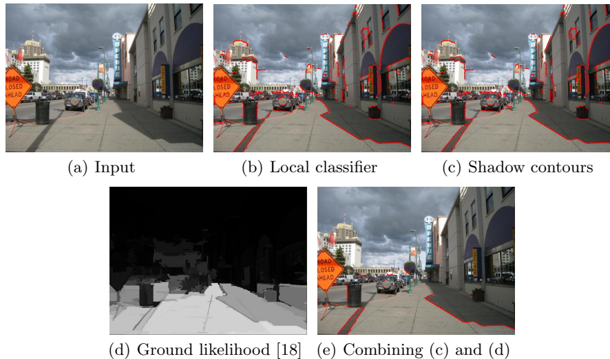
Fig. 3. Incorporating scene layout for detecting cast shadows on the ground. Applying our shadow detector on a complex input image (a) yields false detections in the vertical structures because of complex effects like occlusion boundaries, self-shadowing, etc. (b) & (c). Recent work in scene layout extraction from single images [18] can be used to estimate the location of the ground pixels (d). We show how we can combine scene layout information with our shadow contour classifier to automatically detect cast shadows on the ground (e).
