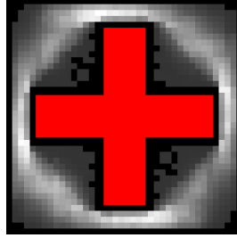
Fig. 9. Coverage over a simple environment. Obstacles are in red; covered areas are in grey. Brighter grey means more coverage (i.e., the grid location is covered by more clips).
