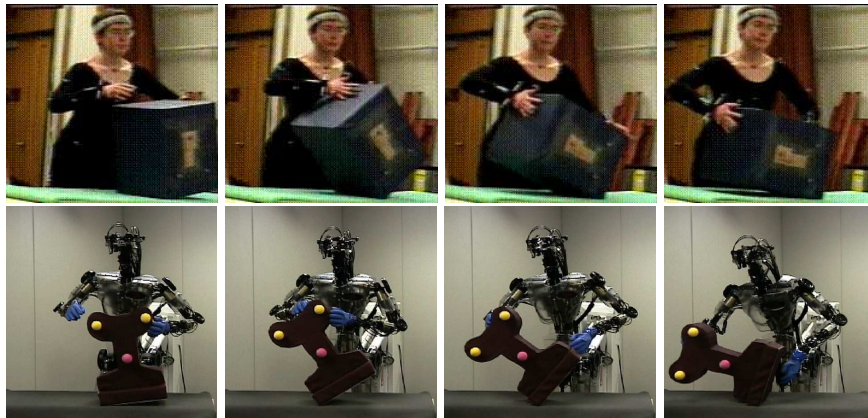
Fig. 1. (Top) Human demonstration of a tumbling task. (Bottom) The demonstration has been adapted to a new object geometry and to the robot kinematics.
