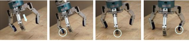
Fig. 6: Compliant finger landing sequence: the circles indicate which new finger has made contact with the support surface.
