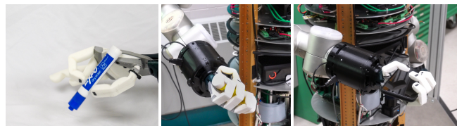
Fig. 1. Soft hand design fully printed from flexible TPU-filament performing a variety of grasps on objects of different shapes, including a precision tripod grasp holding a marker ( left ), a power grasp holding a glue stick ( center ), and a smartphone ( right ). The hand design is self-contained including motors and can be mounted to any robot arm or humanoid robot such as the CMU-Ballbot [17].
