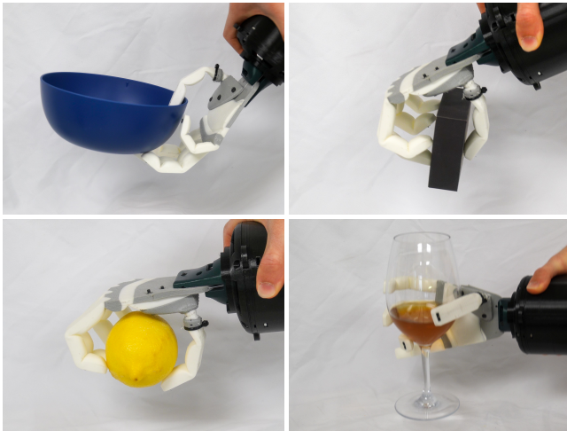
Fig. 11. Based on the results in the design study shown in Figure 10, candidate (d) is selected for fabrication. All grasps are successfully completed in a pick and place setup using key-framed open-loop poses that match the results obtained in our simulation.
