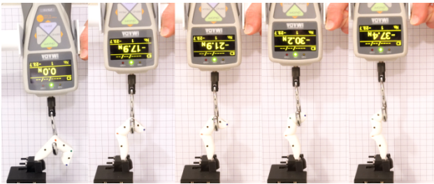
Fig. 8. Individual finger strength test: In the flexed configuration, the finger withstands a maximum load of 37.4N before slipping. No visible damage to the finger was observed when examining the finger after the test.
