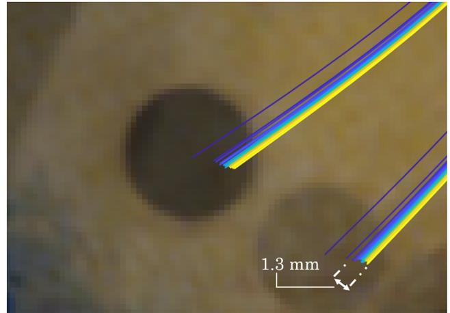
Fig. 6. The fingertip position was observed to drift (shown as blue to yellow) over 8000 grasps.
