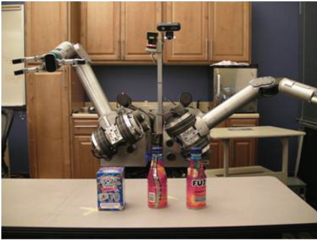
Fig. 4. The HERB robot and the objects (Pop Tarts and Fuze Bottle) used in the test. The objects are fully filled with contents.
