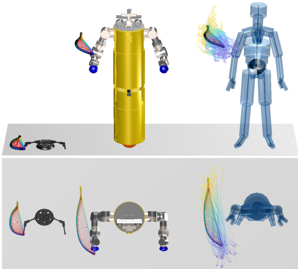
Fig. 8. Pushing skill model transfer from human to robots, for the example of a 0^\circ - 45^\circ push at walking speed: We fit the pushing skill model to the data captured in our MoCap study. The original human trajectories for this push are shown as partially transparent lines next to the human model (right), the resulting model is highlighted in solid color. The skill model is transferred to the Ballbot (center), and the PushBot (left). Trajectories are shifted w.r.t. the CoM of the different embodiments, and scaled to lie within arm workspace.
