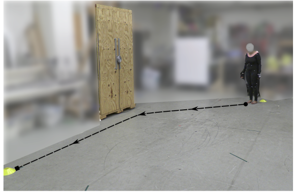
Fig. 2. Motion capture setup: Study participants wear a full-body suit with markers that are tracked by a Vicon motion capture system. A wall-mounted force-torque sensor is used to record reaction forces and cones are placed at the respective entry and exit angles for visual guidance during the motion.
