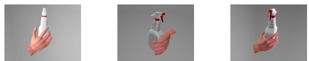
Fig. 9. Three phone grasp candidates for the spraybottle. The metrics are different because of the different contact points and hand orientation.
