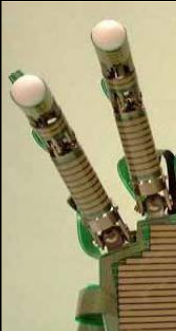
Force sensing resistor technology
