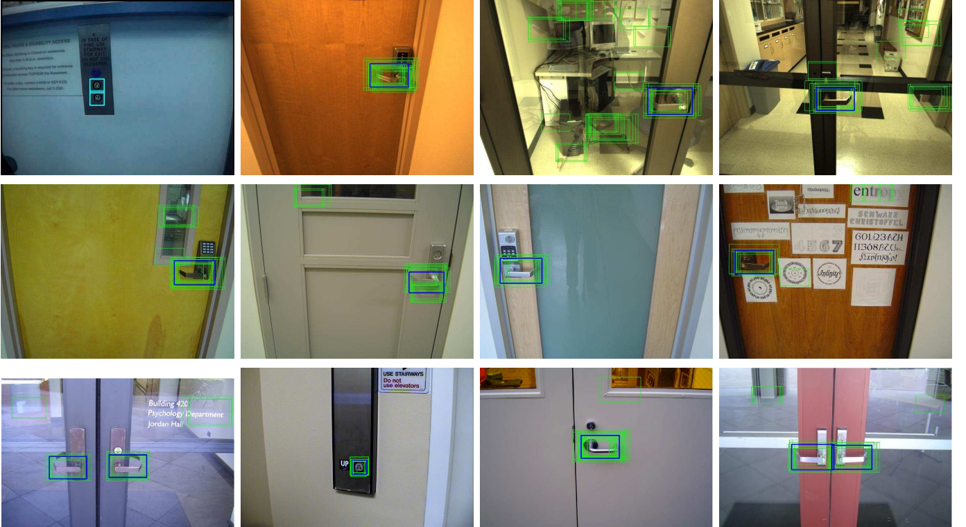
Fig. 3. Results on test set. The green rectangles show the raw output from the classifiers, and the blue rectangle is the one after applying context.
