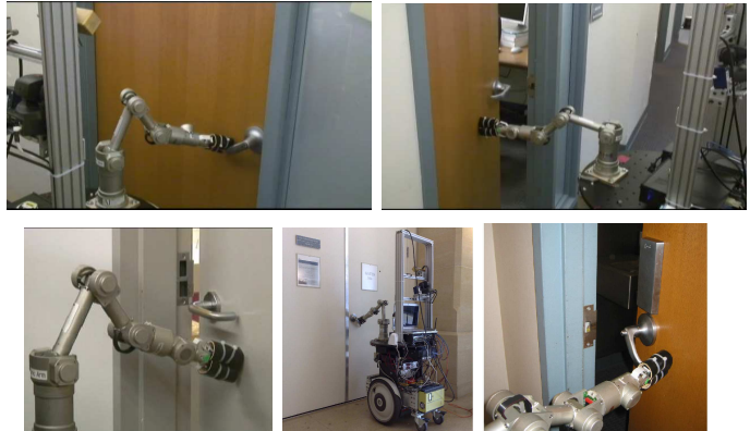
Fig. 7. Some experimental snapshots showing our robot opening different types of doors.
