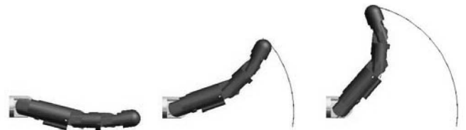
Fig. 18. Three ADAMS snapshots of the underactuated optimized finger showing the tip trajectory in three different time instants.
