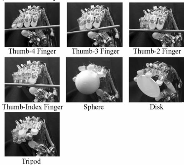
Fig. 11 Result of grasping experiment based on Cutkosky's taxonomy [12]
