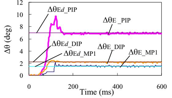
Fig. 9 Response of  $\Delta\theta_E$  in force control experiment
