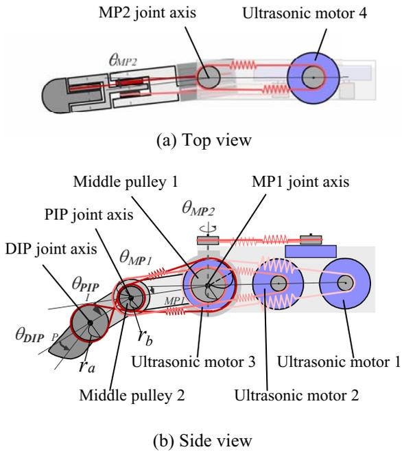
Fig. 3 Outline of driving mechanism of fingers
