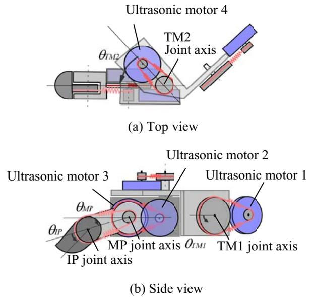
Fig. 4 Outline of driving mechanism of thumb
