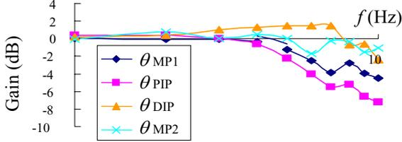
Fig. 8 Frequency response of robot index finger
