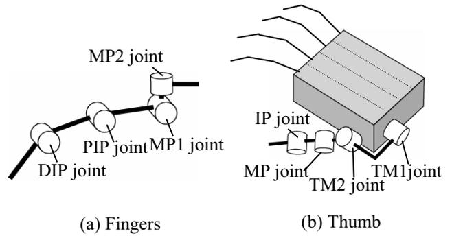
Fig. 2 Arrangement of DOF
