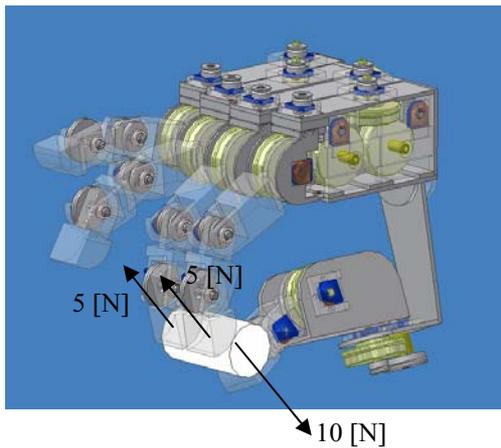
Fig. 5 Reaction force of robot fingers
