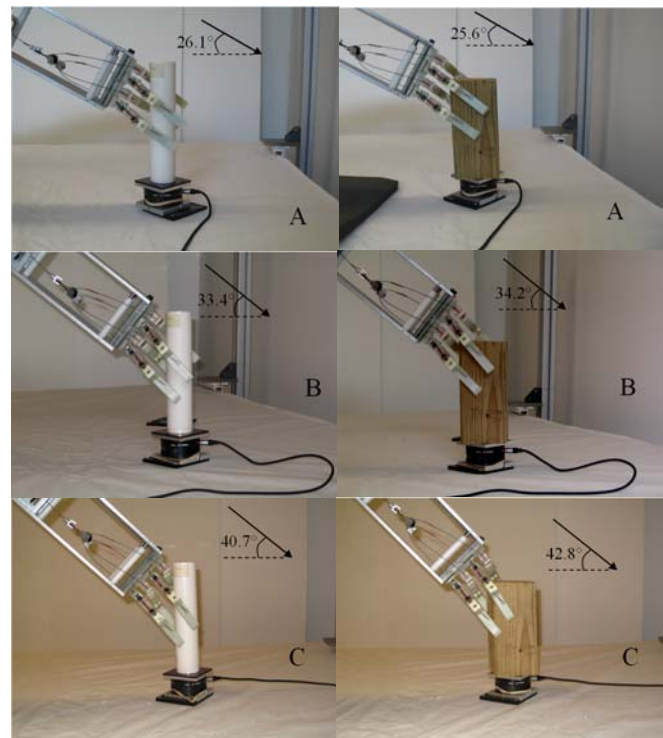
Fig. 9. Two target objects (PVC cylinder with radius 24 mm and wood block with square cross-section 90 mm side length) at three locations (A, B, and C). Note the differences in approach angle for the locations, the main factor affecting the force and grasp space results.
