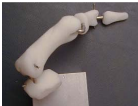
Figure 4. Assembly of bones and link arms. Note that the pins used are larger than in the final design for visibility of the joint axes.
