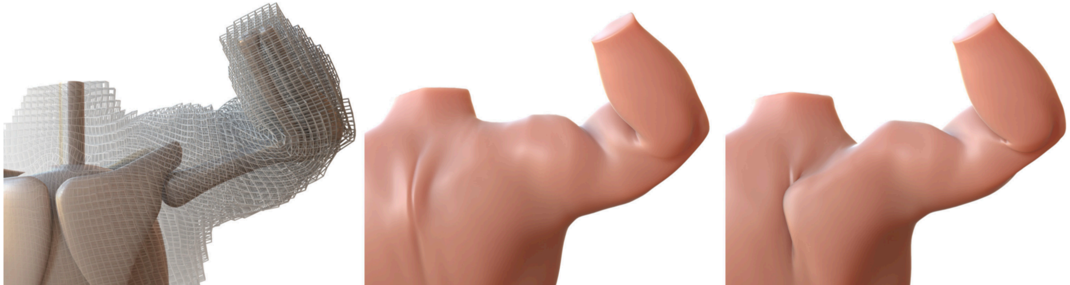
Fig. 1. Left: Thirteen skeletal bones drive a hexahedral lattice with 45,809 elements and 156,078 degrees of freedom. Center: A quasi-static simulation with our new Neo-Hookean model and a Poisson's ratio of \nu = 0.488 . Wrinkles and bulges emerge from our model's excellent volume-preserving properties. An average time step with our model took 13.7 Newton iterations, 5,860 Conjugate Gradient (CG) iterations, and 25.6 seconds. Right: The same simulation with corotational elasticity and \nu = 0.488 . The model fails to preserve volume and instead collapses the trapezius and forms a spurious fold around the shoulder blade. The artifacts persist across all values of \nu . An average time step with this model took 17.9 Newton iterations, 16,183 CG iterations, and 46.6 seconds. ©Disney/Pixar.
