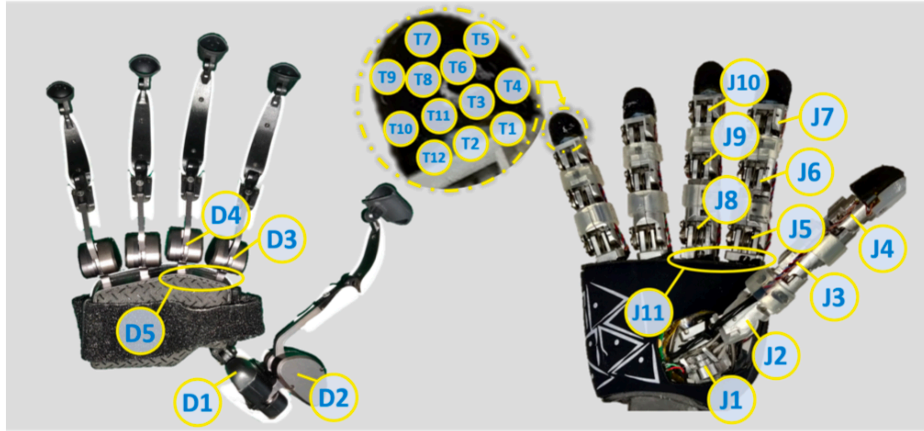
Fig. 3: The anthropomorphic haptic device and the iCub 's hand. Left: Dexmo . D_1 - D_5 are the joints for controlling iCub . Right: iCub . J_1 - J_{11} : the controlled joints. J_4, J_7, J_{10} are coupled with J_3, J_6, J_9 respectively. Each fingertip is equipped with 12 tactile sensors ( T_1 - T_{12} ) arranged as shown.
