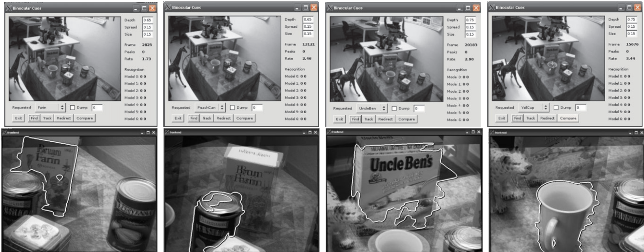
Fig. 18. The visual front end. The top row shows the wide-field view where the visual search selection is made. The bottom row shows the foveal view in which the binocular segmentation and recognition as well as validation is performed.
