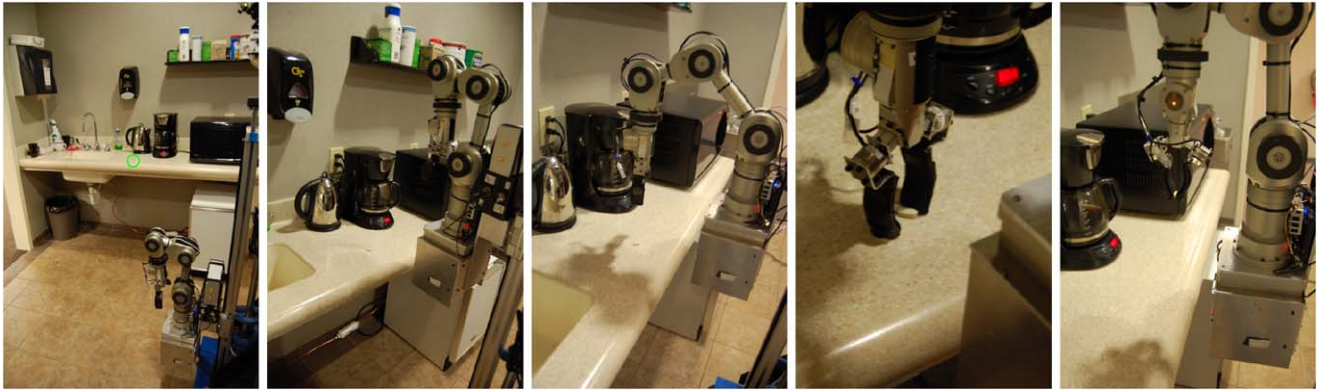
Fig. 4 These images are from one of the experiments that we performed to evaluate the performance of the robot (Sect. 5.1). The robot picks up a pill from a kitchen counter top after the user briefly illuminates the pill with a laser pointer. The first image shows the starting
