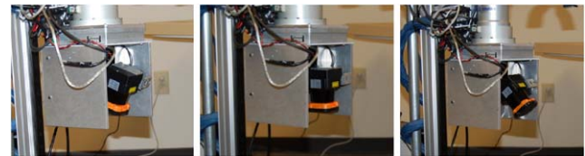
Fig. 3 This figure shows the servo tilting the laser range finder to generate a 3D point cloud
