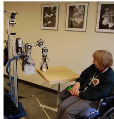
Fig. 1 The mobile manipulator, EL-E, delivering an object to a table after the patient briefly illuminated it with a laser pointer (image used with permission and IRB approval)
