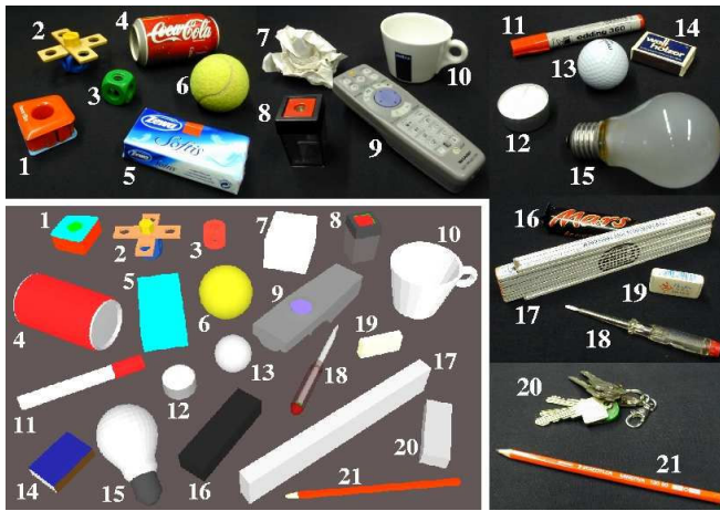
Fig. 7. Set of benchmark objects and their 3D-models in simulation used to evaluate the grasp strategy and the grasps before and after optimization.
