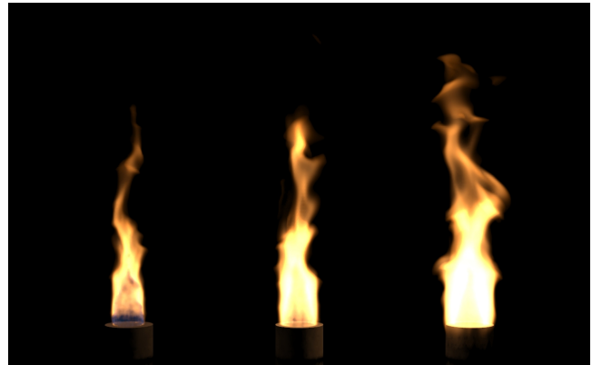
Figure 7: Comparison of flame shapes for differing degrees of gaseous expansion. The amount of expansion increases from left to right making the flame appear fuller and more turbulent.
