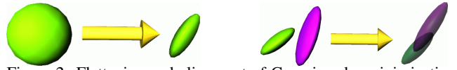
Figure 2: Flattening and alignment of Gaussians by minimization of entropy and cross-entropy, respectively. Gaussian distributions are visualized as ellipsoid iso-probability contours.
