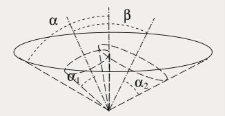
Figure 2: Cone (angle  $\alpha$ ) enclosing its two "descendant" cones in the hierarchical tree (angles  $\alpha_1$  and  $\alpha_2$ ).
