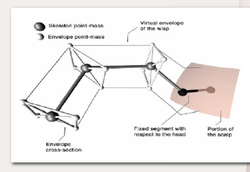
Figure 2.2: Elements defining a deformable volumetric wisp [PCP01a].
