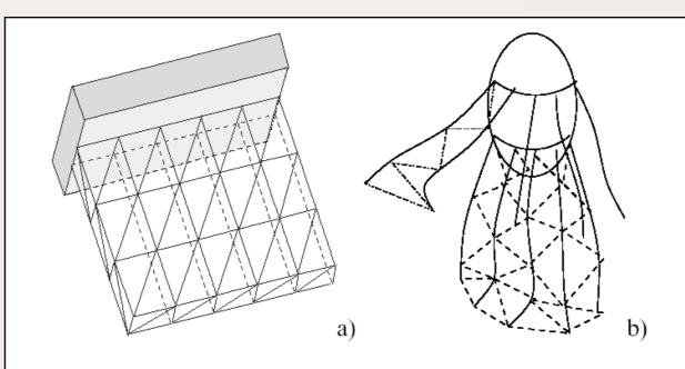
Figure 3: a) For a brush, triangle strips can be inserted between horizontally and vertically adjacent guide hairs. b) For a human scalp, triangle strips are inserted only between horizontally adjacent guide hairs
