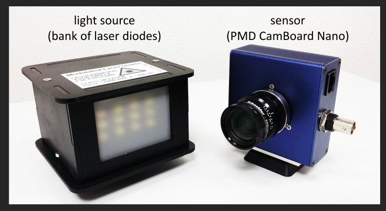
Maximum System Modulation Frequency = 125 MHz.
