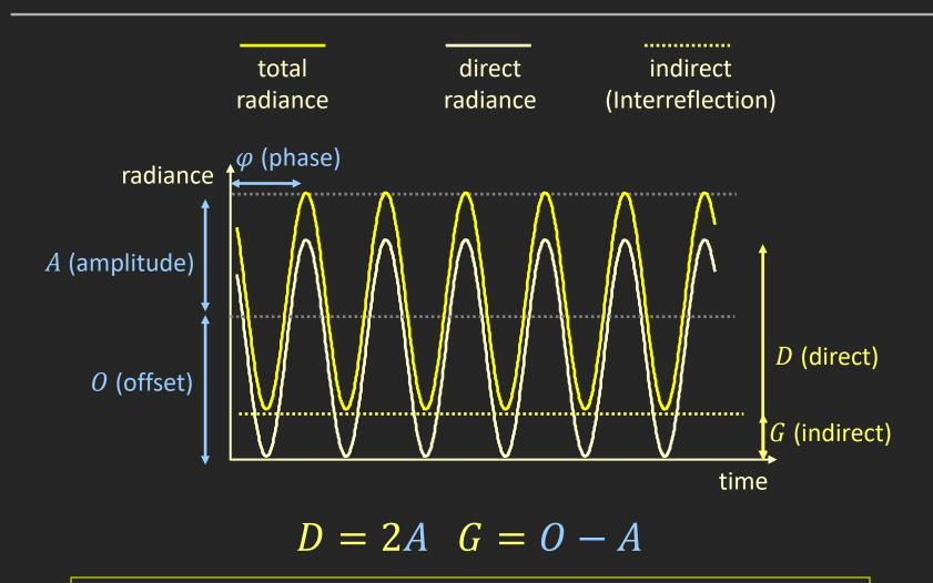
**Direct-Indirect Separation Using Three Measurements**
