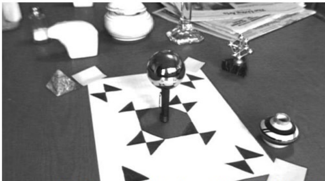
(b) Camera calibration grid and light probe
