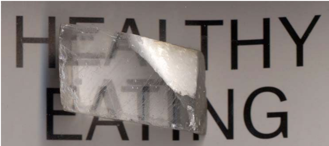
birefringence in a calcite crystal
