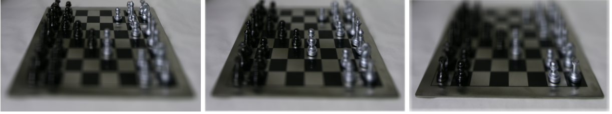
Figure 3: Refocusing at different depths using the largest aperture. The left image corresponds to using Equation (2) with d = 0 (or equivalently, using Equation (1)). These images have had their exposure adjusted to match that of the images in Figure 2, by dividing the result of Equation (2) by the size of the aperture.
