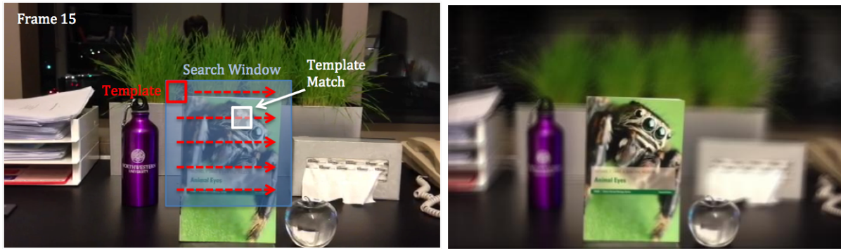
Figure 7: Focusing by template matching. Left: Template matching procedure for one frame. Right: Refocusing result.
