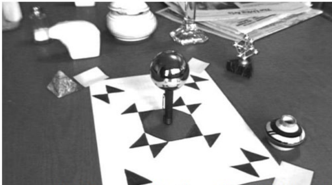
(b) Camera calibration grid and light probe
