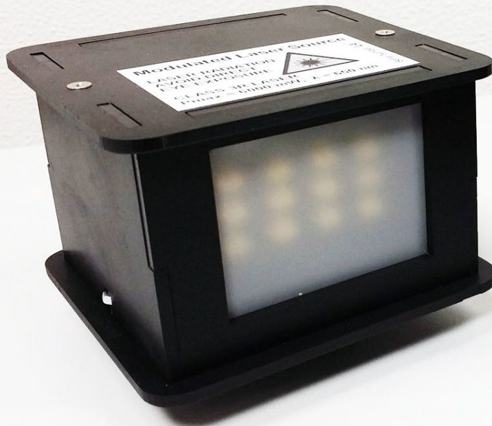
light source (bank of laser diodes)
