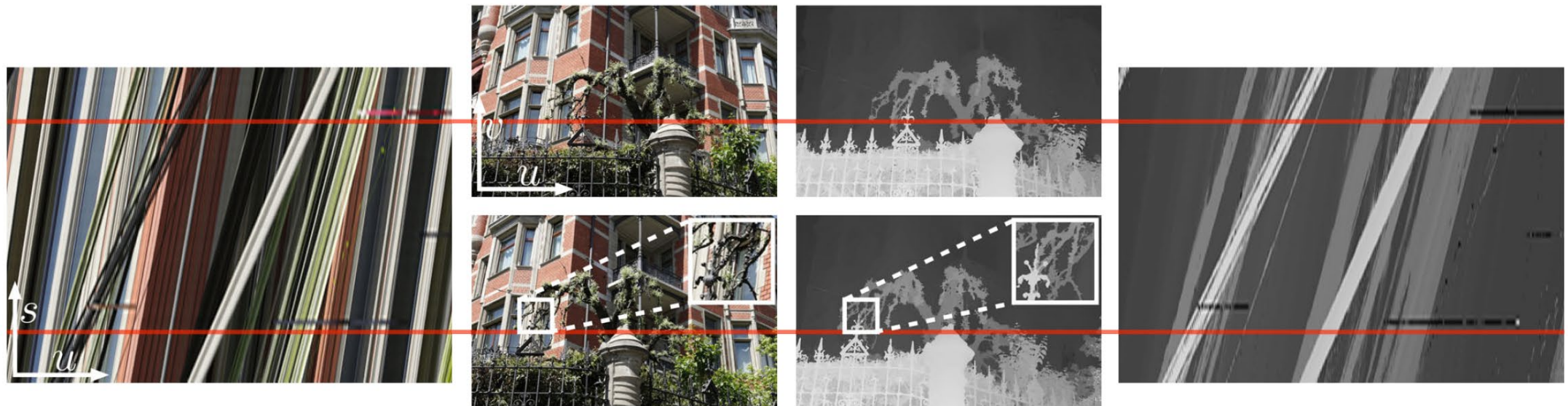
Figure 1: Our method reconstructs accurate depth from light fields of complex scenes. The images on the left show a 2D slice of a 3D input light field, a so called epipolar-plane image (EPI), and two out of one hundred 21 megapixel images that were used to construct the light field. Our method computes 3D depth information for all visible scene points, illustrated by the depth EPI on the right. From this representation, individual depth maps or segmentation masks for any of the input views can be extracted as well as other representations like 3D point clouds. The horizontal red lines connect corresponding scanlines in the images with their respective position in the EPI.
