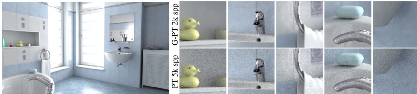
Figure 1: Comparing gradient-domain path tracing (G-PT, L_1 reconstruction) to path tracing at equal rendering time (2 hours). In this time, G-PT draws about 2,000 samples per pixel and the path tracer about 5,000. G-PT consistently outperforms path tracing, with the rare exception of some highly specular objects. Our frequency analysis explains why G-PT outperforms conventional path tracing.
