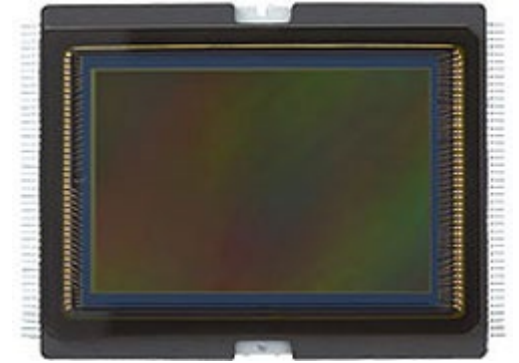
Canon 6D sensor (20.20 MP, full-frame)
