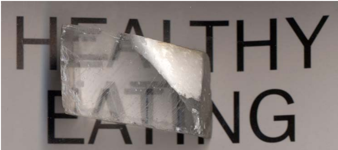
birefringence in a calcite crystal
