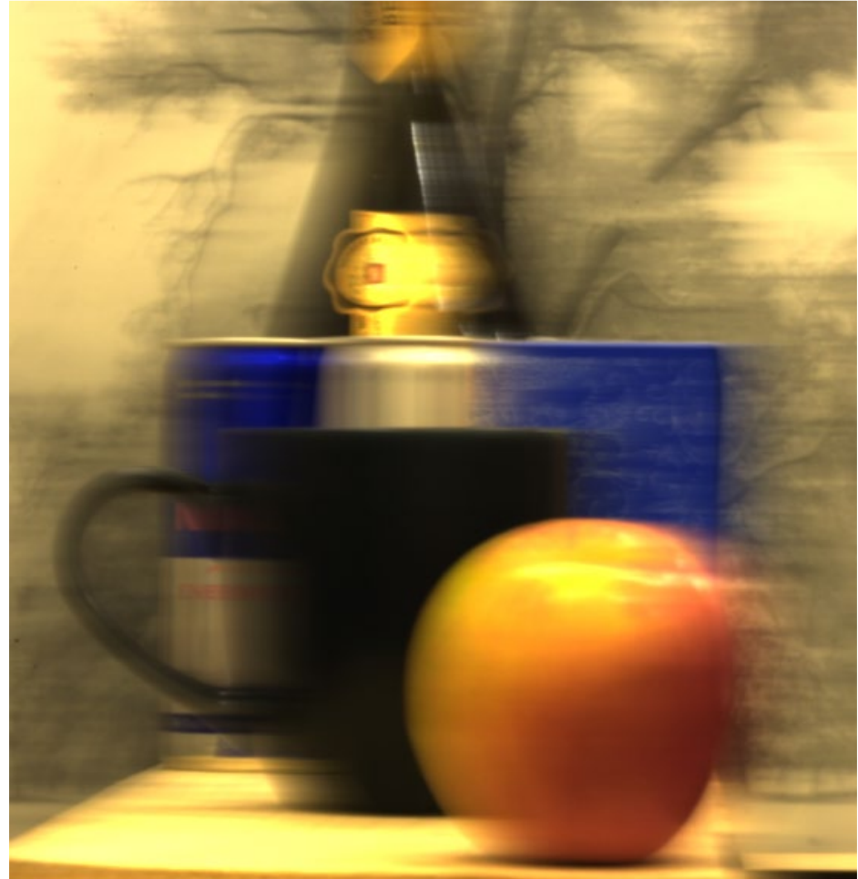
parabolic input - blur is invariant to velocity
