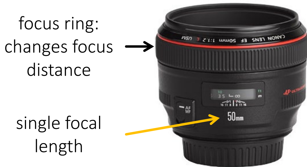
Prime lens: fixed focal length
