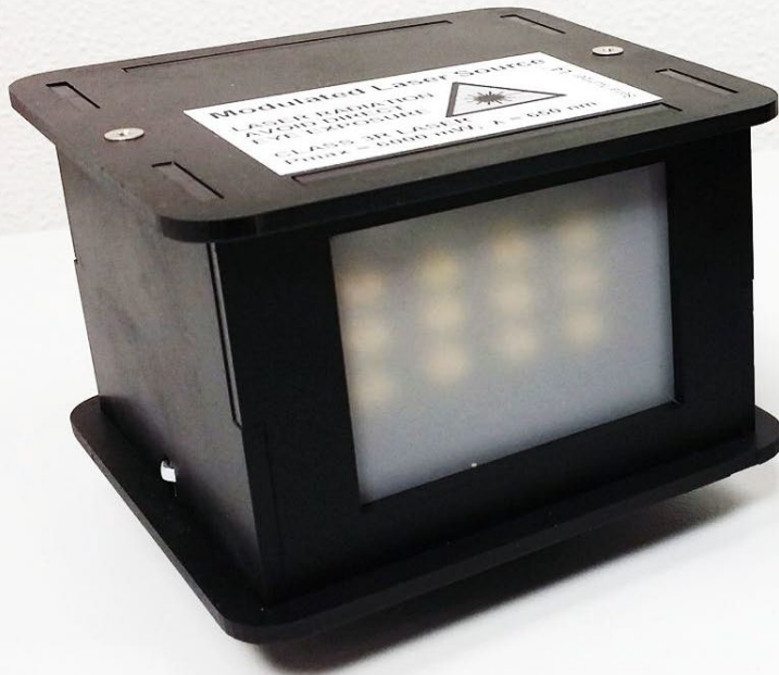
light source (bank of laser diodes)
