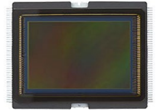
Canon 6D sensor (20.20 MP, full-frame)
