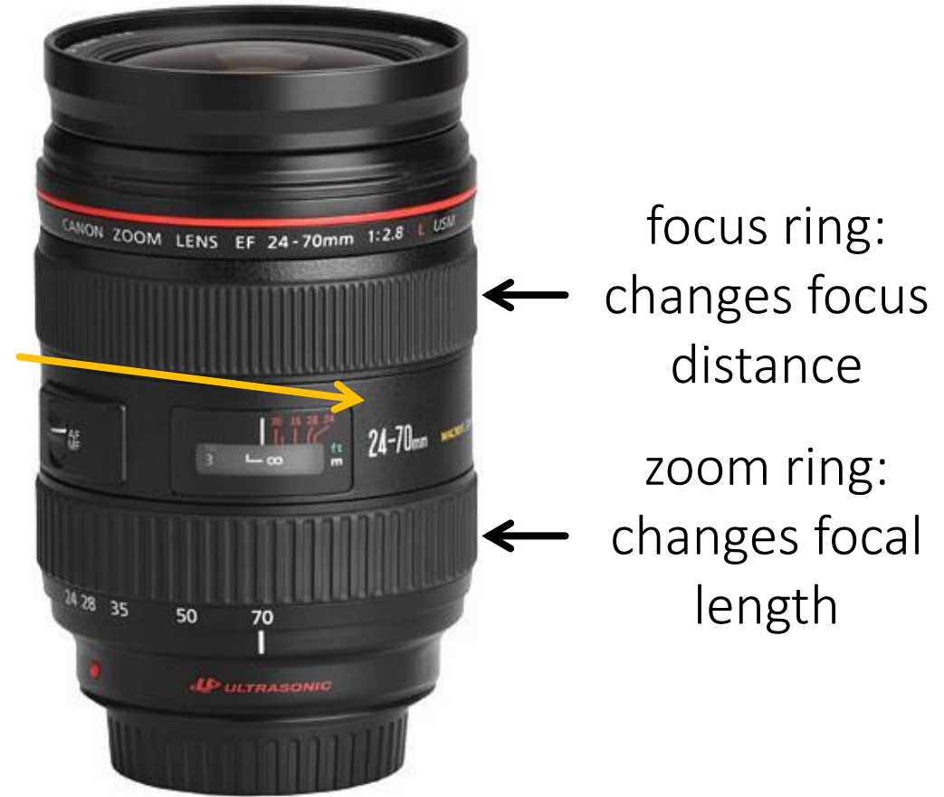
Zoom lens: variable focal length
