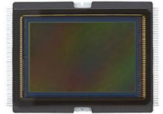
Canon 6D sensor (20.20 MP, full-frame)
