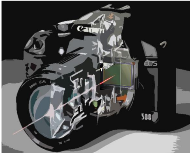
digital sensor to capture focused light (electrical process)
