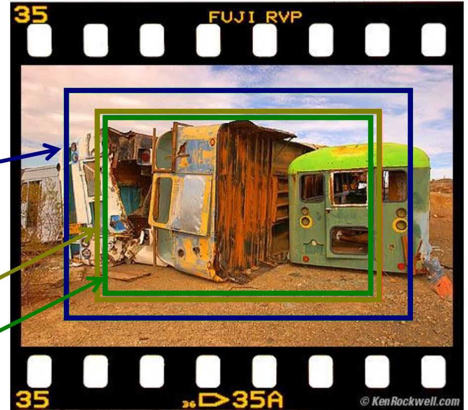
How much field of view is cropped when using a sensor smaller than full frame.
