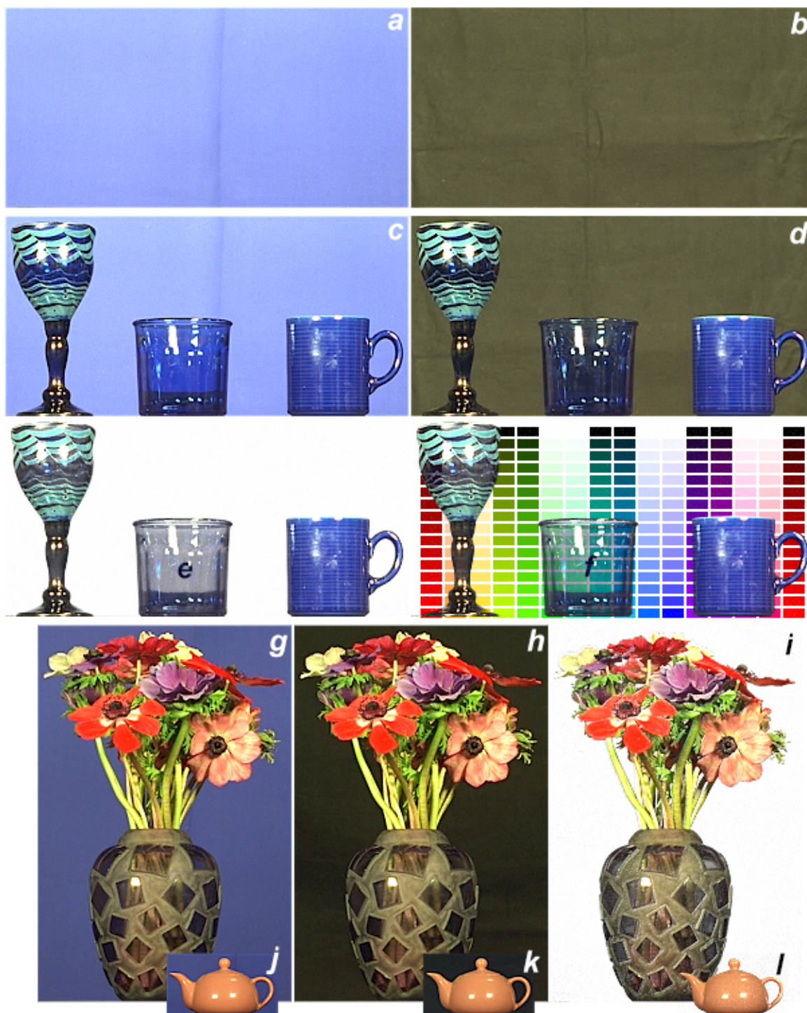
Figure 2. Practical triangulation matting. (a-b) Two different backings. (c-d) Objects against the backings. (e) Pulled. (f) New composite. (g-i) and (j-l) Same triangulation process applied to two other objects (backing shots not shown). (l) Object composited over another. The table and other extraneous equipment have been “garbage matted” from the shots. See Fig. 5.
